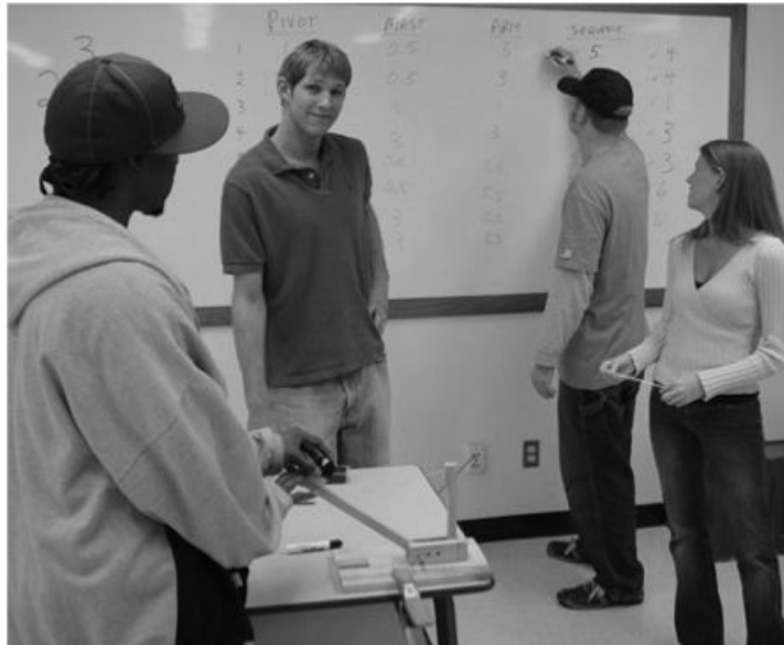
Students running a 2^3 full-factorial-designed experiment to optimize the settings on the catapult to maximize the distance that the ball is thrown. [Exercise 1]
