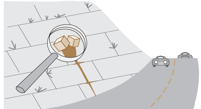
Figure 7.16 Geochemistry from a car window. Oxidation of pyrite within this limestone has left a tell-tale streak of red hematite. The sulfuric acid has either evaporated or gone into the nearest creek.
